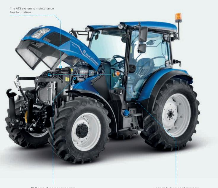
All the maintenance can be done on one side, all service points are on the left side of the engine to make routine servicing easier
